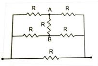
By symmetry, points A and B are at the same potential. Thus, removing the resistance R between A and B, the circuit reduces to three resistances of 2R, 2R and R in parallel.
